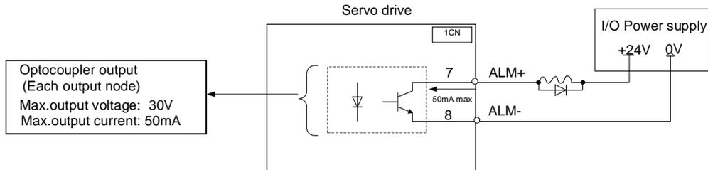
External +24V I/O power supply is required, since there is no +24V power supply available inside servo drive.
