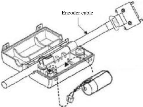
C. Cover the shell of the battery case.
