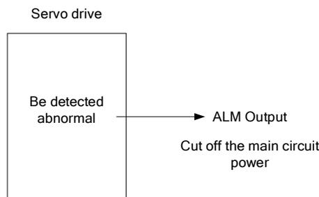
Normally, the external circuit consists of /ALM should be able to switch off power of servo drive.
