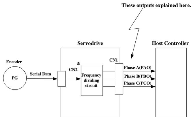
\* The dividing output phase form is the same as the standard setting(Pn001.0=0) even if in the reverse rotation mode(Pn001.0=1).
