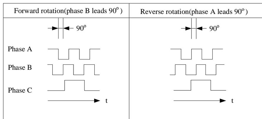
If a servomotor is not equipped with the absolute encoder, servomotor needs two circles rotation before using the servodrive's phase-C pulse output for zero point reference.
