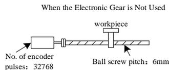
To move a workpiece 10mm :
