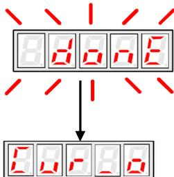
5. Press the ENTER key to return to the utility function mode display Fn005.
