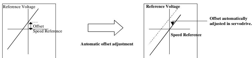
After completion of the automatic adjustment, the amount of offset is stored in the servo drive. The amount of offset can be checked in the speed reference offset manual adjustment mode (Fn004). Refer to **4.5.3 (2) Manual Adjustment of the Speed Reference Offset**.
