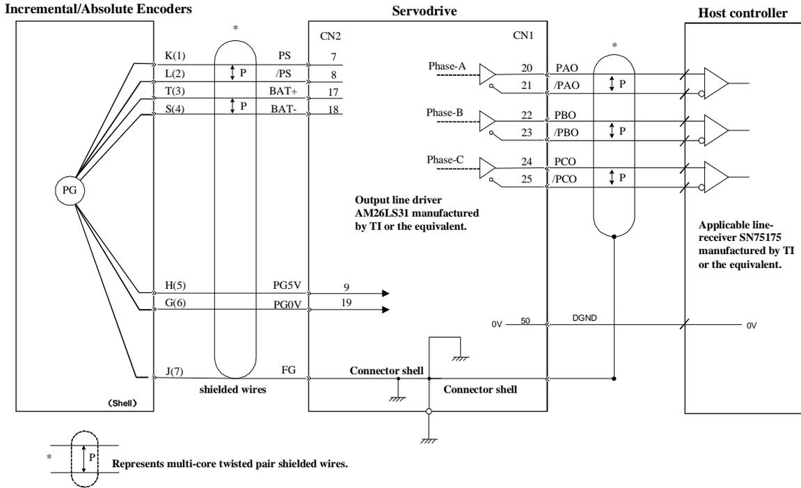
Note: (1) There are no BAT+ and BAT- signals in incremental encoder.
