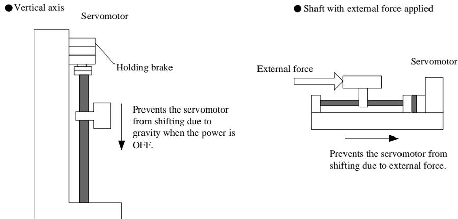
1. The brake built into the servomotor with brakes is a deenergization brake, which is used to hold and cannot be used for braking. Use the holding brake only to hold a stopped servomotor.
