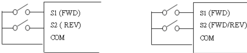
Figure 4-4 Terminal Board Drive Operation Modes
