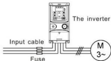
Figure 3-11 Fuse configuration
