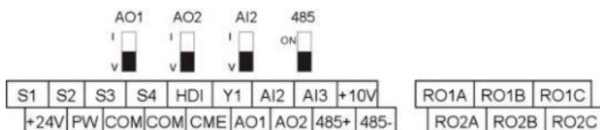
Figure 3-7 Terminals of control circuit
