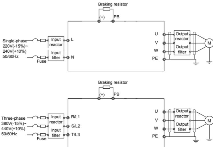
Figure 3-3 Connection diagram of main circuit
