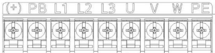
Figure 3-5 3PH terminals of main circuit
