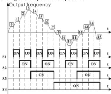
When S1=S2=S3=S4=OFF, the frequency input manner is selected via code P00.06 or P00.07. When all S1=S2=S3=S4 terminals aren't off, it runs at multi-step which takes precedence of keypad, analog value, high-speed pulse, PLC, communication frequency input. Select at most 16 stages speed via the combination code of S1, S2, S3, and S4.
