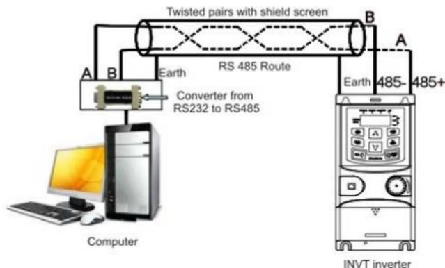
Figure 1 RS485 physical connection in single application
