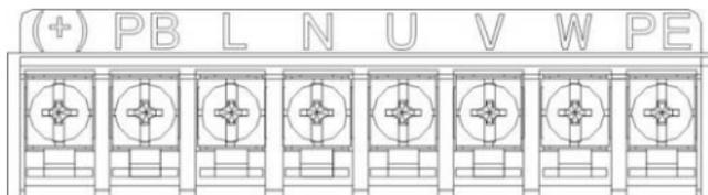
Figure 3-4 1PH terminals of main circuit
